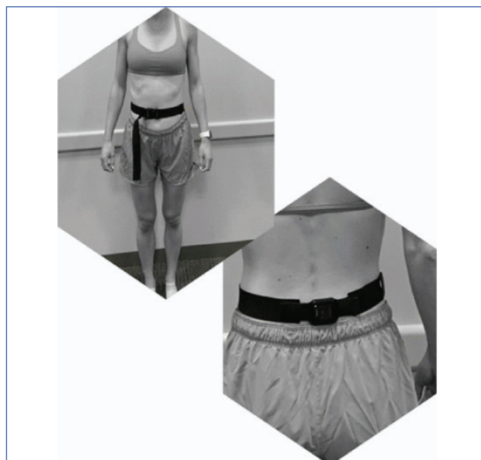
[Table/Fig-1]: Mobility Lab Sensor: Velcro belt with the lumbar accelerometer and gyroscope utilised to measure sway, direction of sway and velocity of sway.
